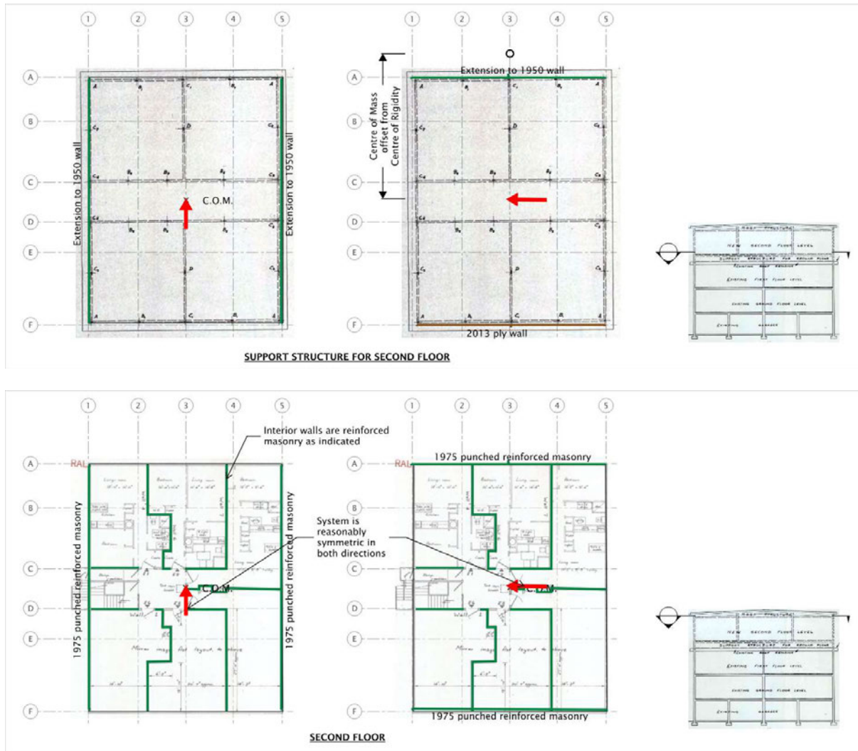
Figure 7: Structural system at each level
