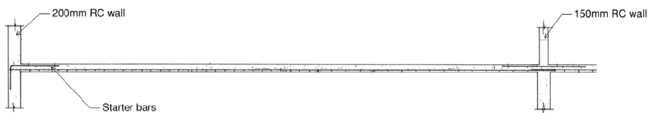
Figure 3.3: Section of typical wall to slab interface
