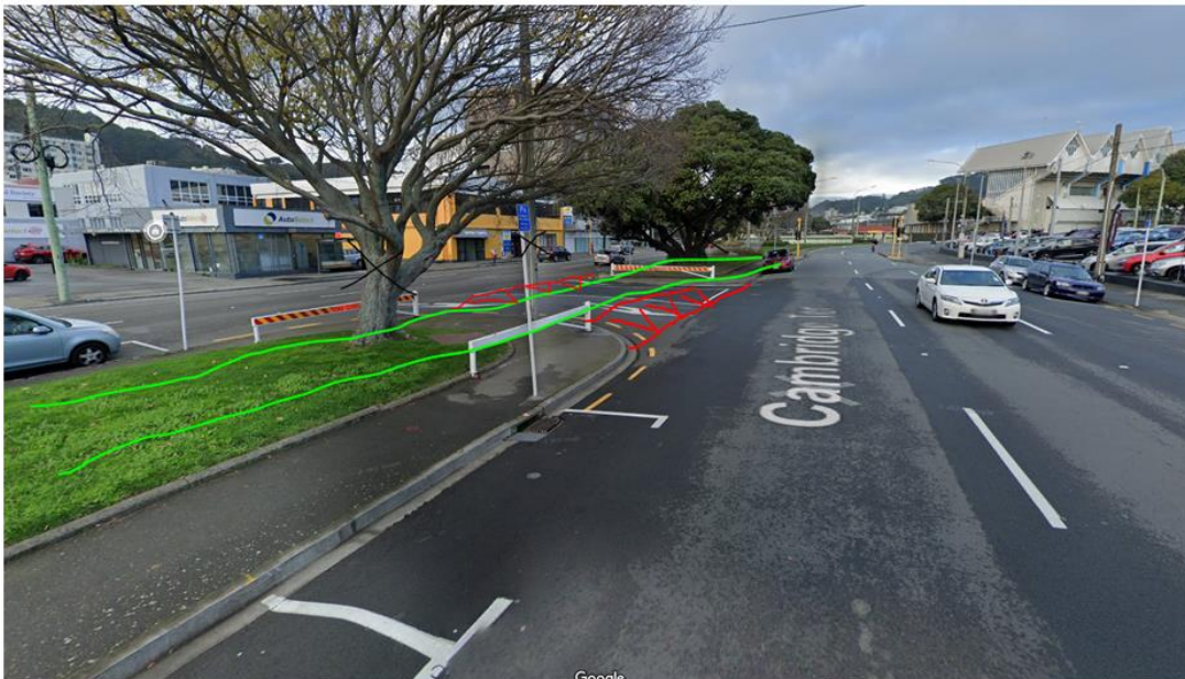
Very rough sketch of raised table for Kent/ Cambridge Tce below, key design consideration would be maximising visibility of cyclists for vehicles and vis versa
