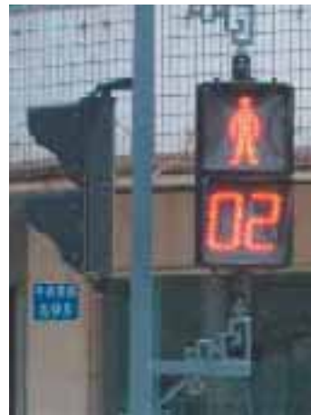
Pedestrian lights informing the pedestrians of extent of waiting /walking periods are frequent in China.
