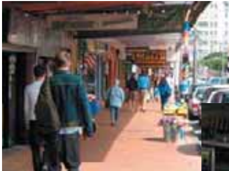
A Attractive Small units, many doors (15-20 units per 100 m) Diversity of functions No closed or passive units Interesting relief in facades Quality materials and refined details
