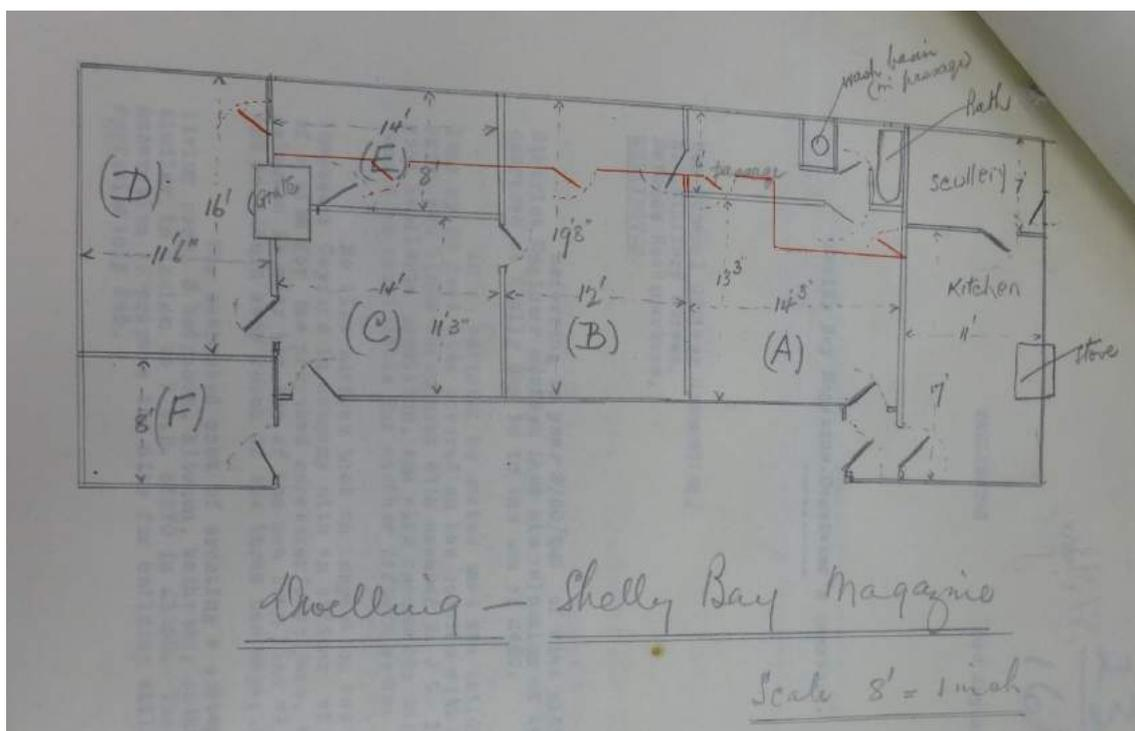
**Fig. 9** Sketch plan showing the Submarine Mining Barracks Building – Caretaker's Quarters in 1925, and the proposed internal alterations to make it suitable for residential purposes.
