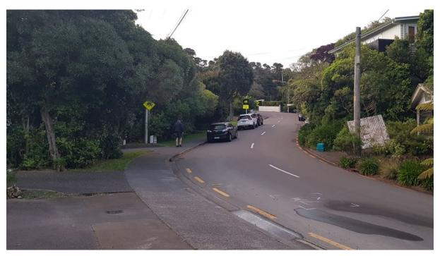
There is greater than 30 m visibility to the east and west satisfying RTS-6 requirements. Again, for completeness, we have also assessed sight distance in accordance with Austroads. The Safe Intersection Sight Distance (SISD) requirement for a 40 km/hr design speed is 73 m. This distance can be satisfied to the north and south.
