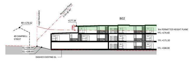
Figure 3: Cross Section showing the relationship between Building B02 and property at 49 Campbell Street
