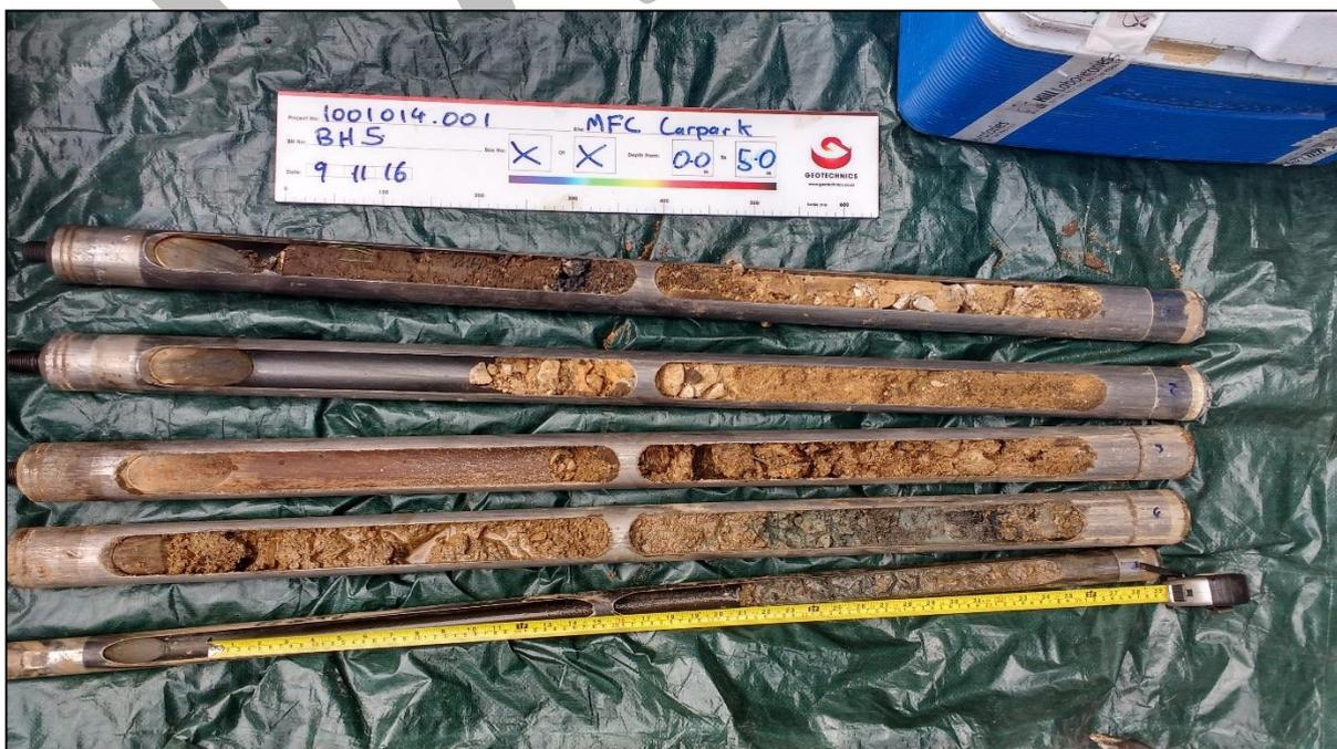
Photograph 5: Recovered core from BH5. Black gravels/slag can be observed at 0.3 m. Photo taken on 9 November 2016. Photo sourced from Geotechnics Limited.
