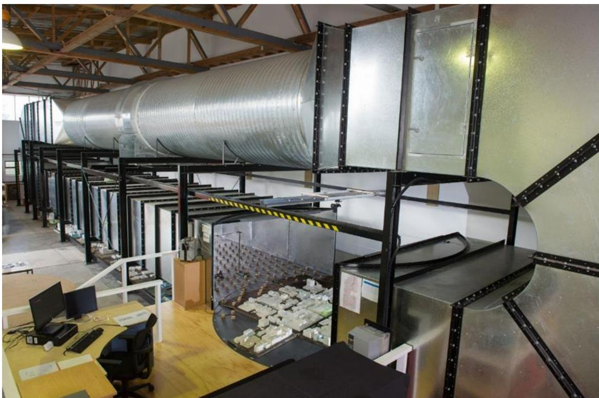
Figure D1: WSP Research and Innovation Centre Wind Tunnel.
