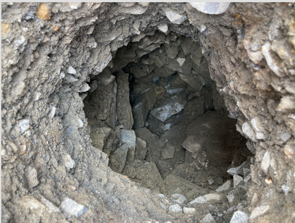
Figure 4 BH101 – Angular cobble/boulder fill in ground
