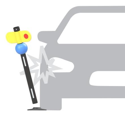
In the inevetable event that Wobly is struck with significant force, the plastic pin easily shears in an attempt to preserve the bollard.
