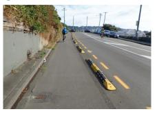
Temporary ground separators which can fit together in various sizes to create a physical gap between bikes and cars.
