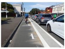
Concrete ground separators which are either keyed into or poured on top of the road surface. These are generally made from a standardised mould.
