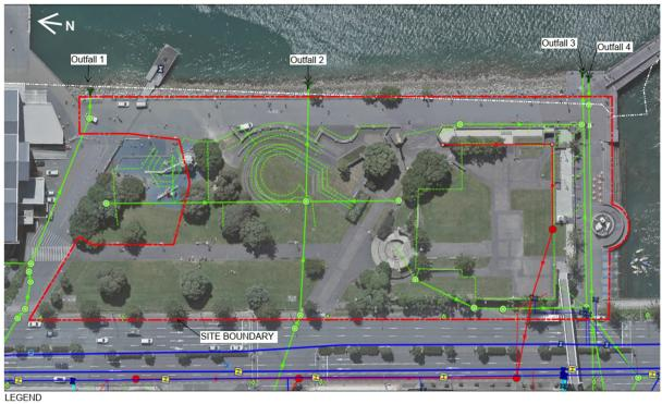
Site boundary — Stormwater pipe ----- Stormwater drain/subsoil — Wastewater pipe ----- Wastewater connection — Water supply pipe — Water supply connection
