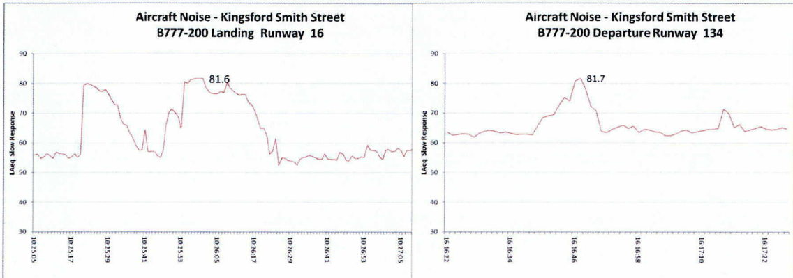
Figure 7 measured B777-200 single event LAFMax sound levels at Wellington Airport, departure runway 34 and an arrival on Runway 16.
