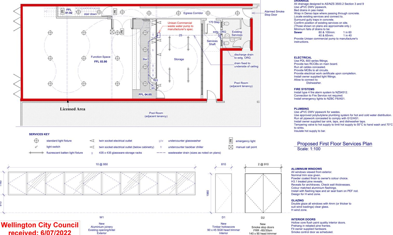
All drainage designed to AS/NZS 3500.2 Section 3 and 9
