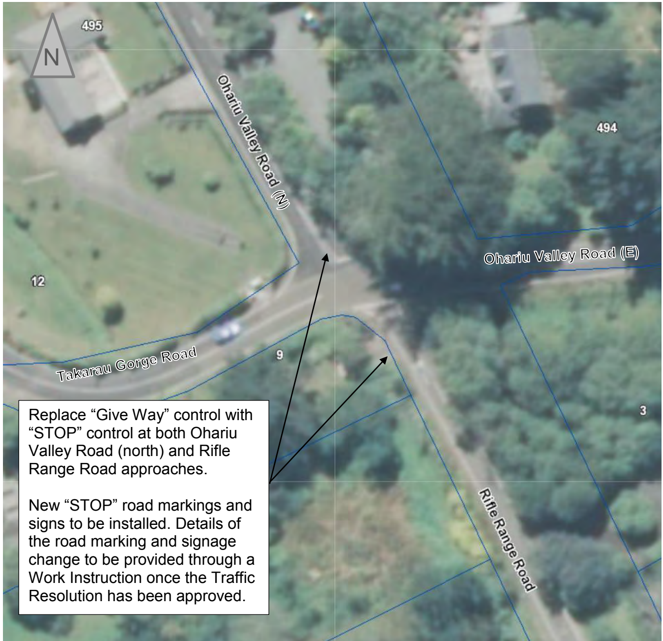
TR17-19 Ohariu Valley Road and Rifle Range Road, Ohariu Valley Proposed Stop Controls
