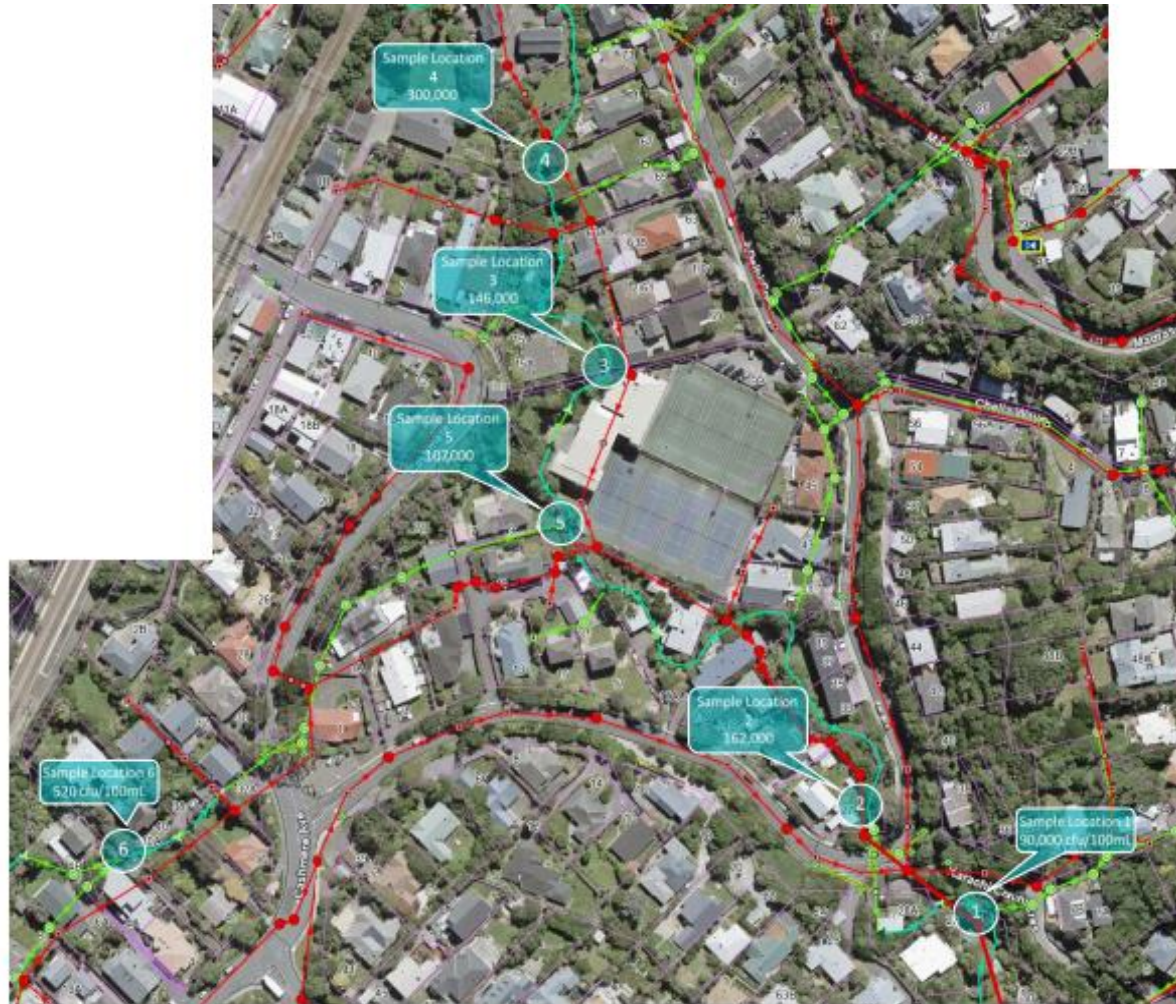
Figure 1. Sampling location and results. The results are measured in Faecal coliforms in cfu/100mL
