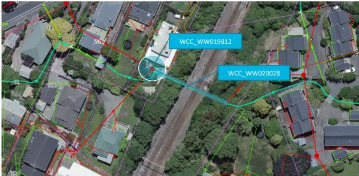
Figure 2. 29 Burma Rd. has a sewer main right next to an open stream. Highlighted are the blocked sewer main the manhole overflow point.
