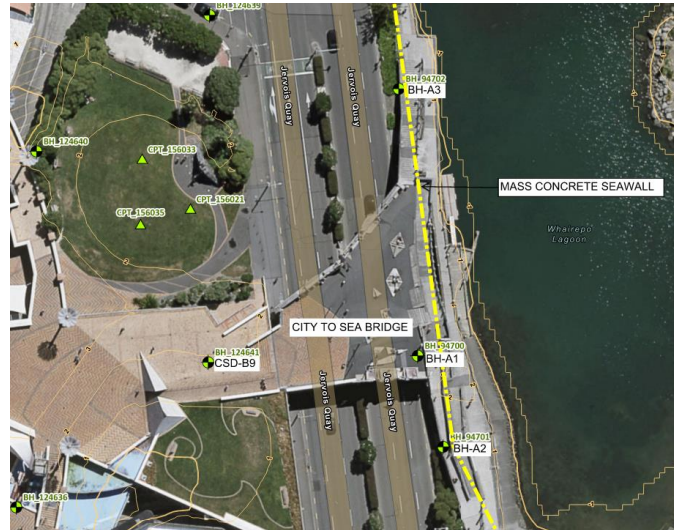
Figure 2-1: Ground Investigation location plan: Source: T+T City to Sea Bridge Geotech Report.
