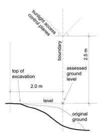
Where the top of the excavation is within 2 metres of the boundary, the assessed ground level at the boundary will be taken from the top of the excavation.
