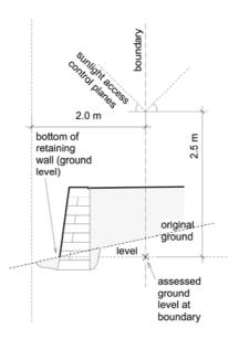
Where the original ground has been raised by earthworks, and the bottom of the earthworks is within 2 metres of the boundary, the assessed ground level at the boundary will be taken from the bottom of the earthworks.
