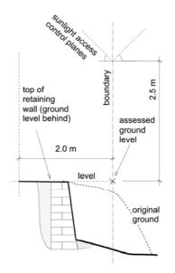
Where the retaining wall supports cut ground, and the ground level behind the top of the retaining wall is within 2 metres of the boundary, the assessed ground level at the boundary will be taken from the ground level behind the top of the retaining wall.
