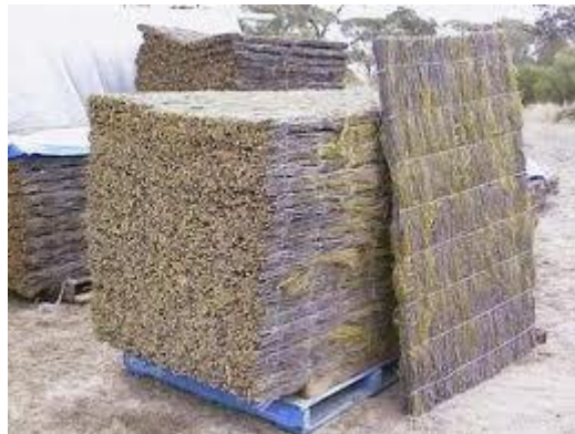
Plate 2: An example of brushwood panels that can be used to create temporary, short-term shade and protection from wind.
