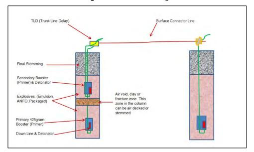
Figure 6: Blast Hole Configuration
