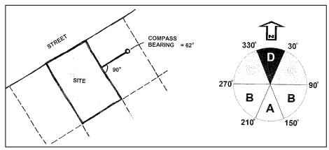
The orientation of a boundary is determined by the compass bearing of a perpendicular line drawn outwards from the boundary. In the example above the compass bearing is  $62^{\circ}$  so the building recession plane angle for Sector C would apply along this boundary.
