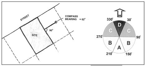
The orientation of a boundary is determined by the compass true north bearing of a perpendicular line drawn outwards from the boundary. In the example above the compass bearing is  $62^{\circ}$  so the building recession plane angle for Sector C would apply along this boundary.
