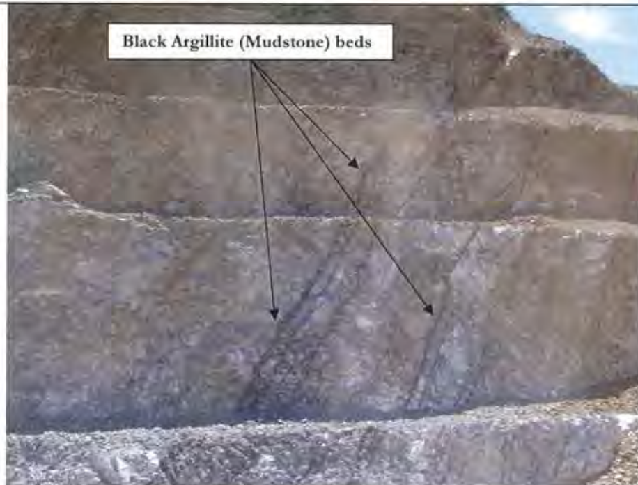
Plate 2 Northern Batter exposing slightly weathered to fresh sandstone dominant greywacke with bedding dipping to the left as defined by black argillite beds.
