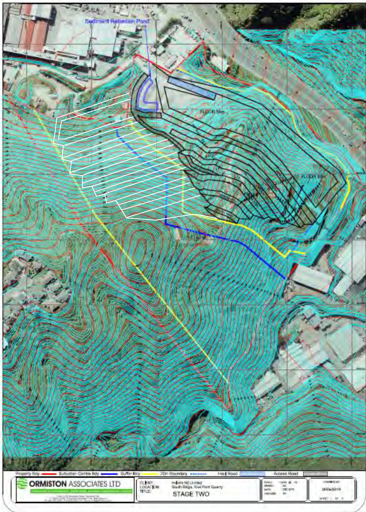
Figure 5: Area 2A expansion option showing indicative benching and pit development (base image source: Ormiston Associates Ltd).
