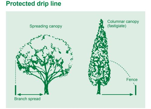
Note: For fastigiate species (erect, almost parallel braches) the tree-protection zone equals half the height of the tree. The actual tree root zone can spread well beyond the canopy drip-line.
